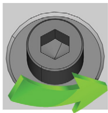
FIG. 28 – SCREWING DOWN THE SCREW TO IMMOBILIZE THE BLOCK
